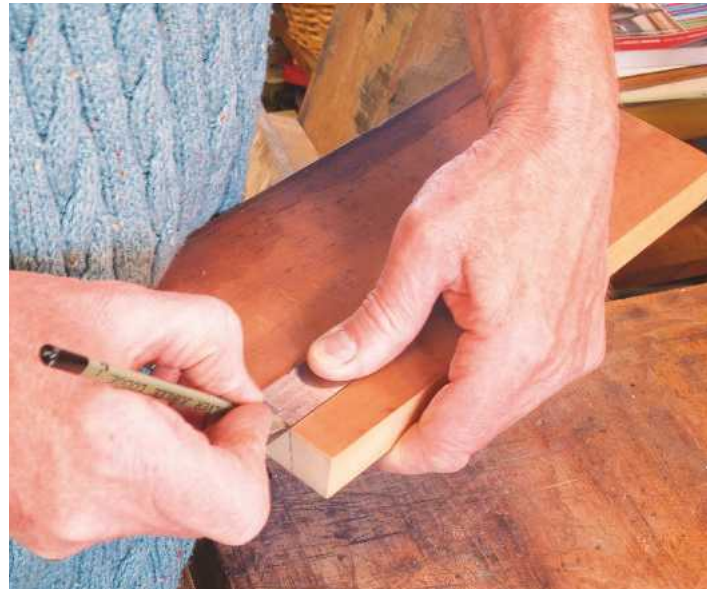
▲ Pic.9 Marking perpendiculars on pin board
